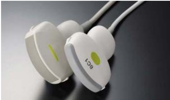
Figure 5 Conventional transducer (left) and thin-convex transducer, PVT-475BT (right) The contact surface of the thin-convex transducer is only 9 mm thick, half that of the conventional transducer.
