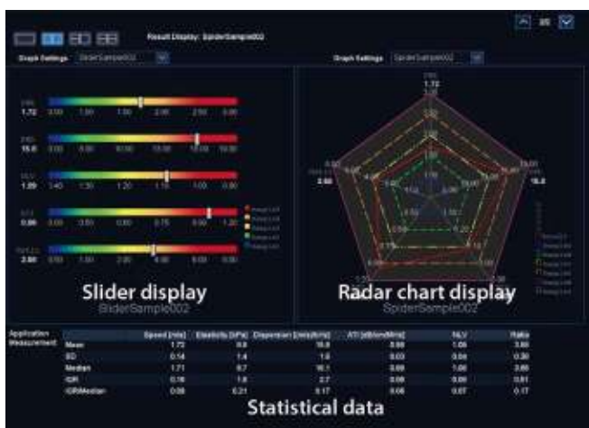
Figure 3 Example of Multi Parametric Worksheet graph display* Sliders (left) and a radar chart can be generated and displayed. * NLV (Normalized Local Variance) and Ratio are W.I.P. functions. The values shown in the figure are only examples.
